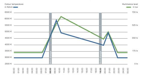
The automatic light identity profile is activated when each shift changes, supporting staff who have just started work with higher light levels and appropriate colour temperatures. These automatic sequences can of course be interrupted and manually adjusted at any point.
